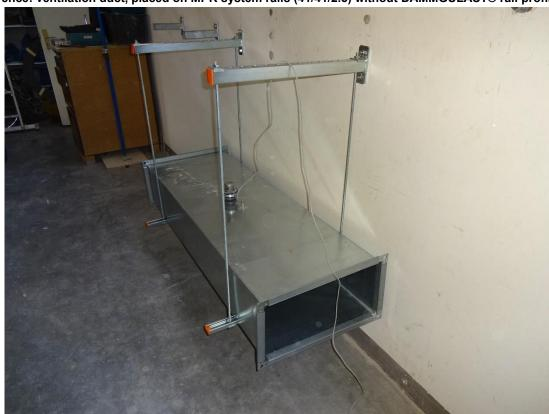
Fig. 2: Reference: ventilation duct, placed on MPR system rails (41/41/2.5) without DÄMMGULAST® rail profiles
