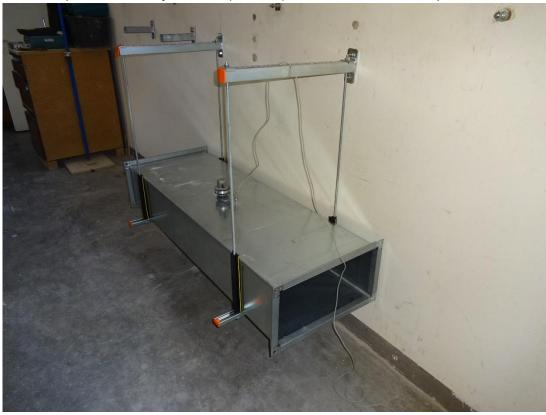
Fig. 4: Ventilation duct, placed on MPR system rails (41/41/2.5) with DÄMMGULAST® rail profiles
